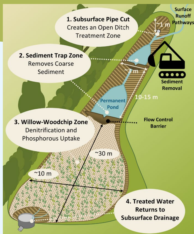
Figure 1: Open-ditch multistage treatment zone schematic illustrating key design principles and associated hydrological processes.
